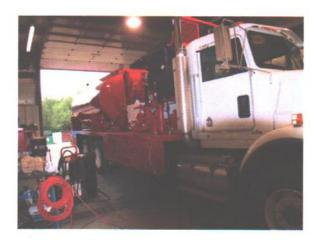
As these units are equipped with a crude storage tank and a 3" load/unload gear pump, they can also perform the same function as a tank truck. However, weight restrictions to the chassis or road regulations may not allow the transport of full capacity volumes.
